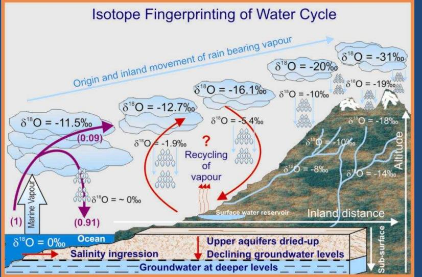
Vapor source region, advancement of vapor front, recycled component, groundwater and snow melt contribution to river etc.
