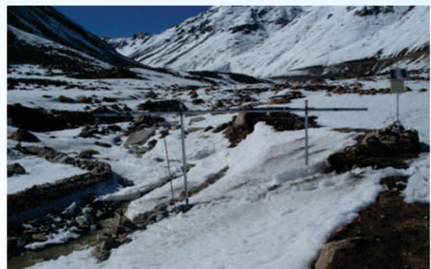
Discharge site equipped with Automatic Radar Water Level recorder (AWLR)
