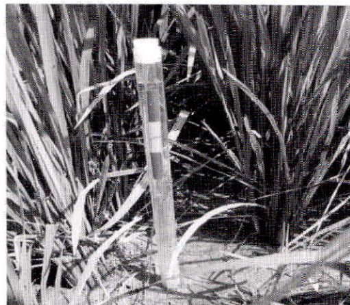
Fig 1: Tensiometer installed for irrigation scheduling
