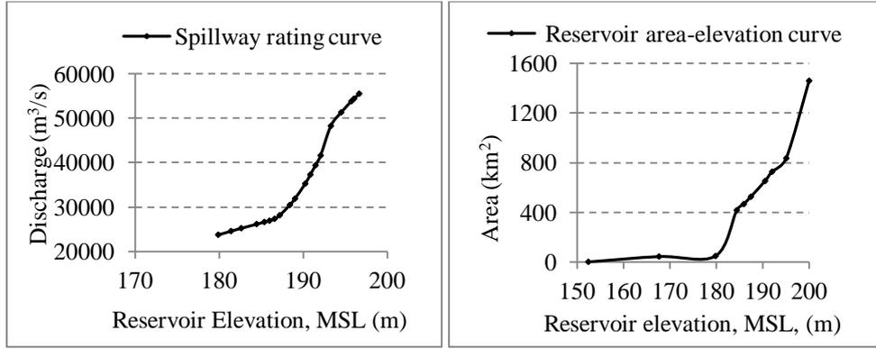
Fig. 2: Spillway Rating Curve
