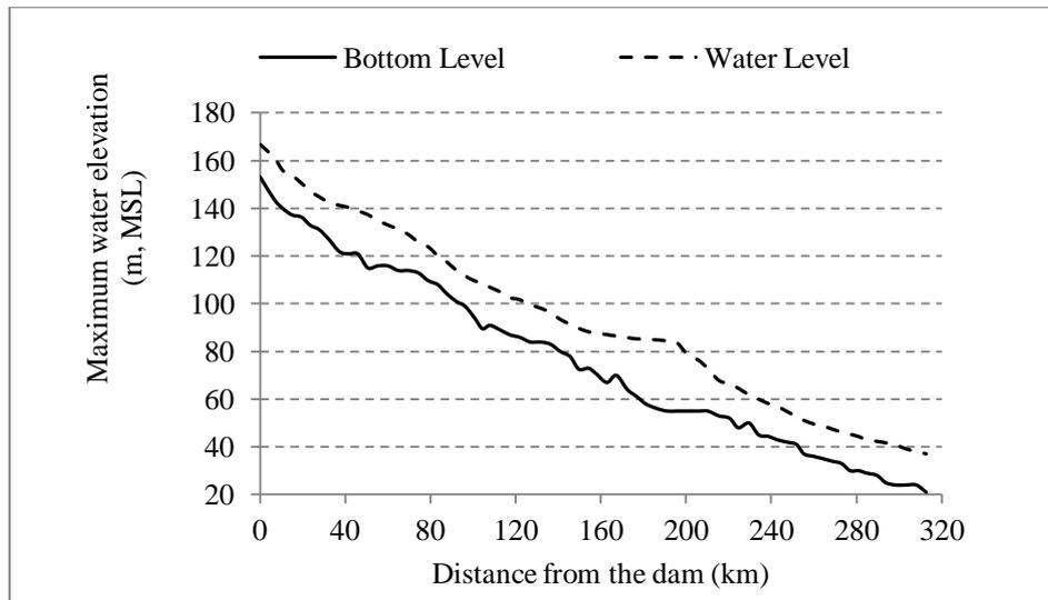
Fig. 6: Maximum Water Elevation Profile at Downstream River Sections
