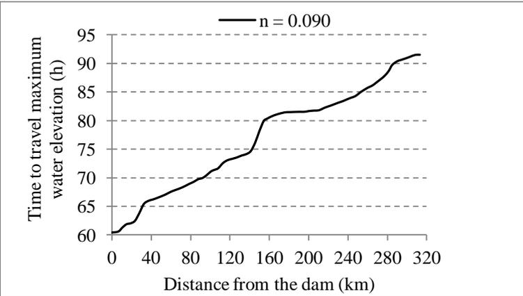
Fig. 8: Time to Travel Maximum Water Elevation at Downstream River Sections
