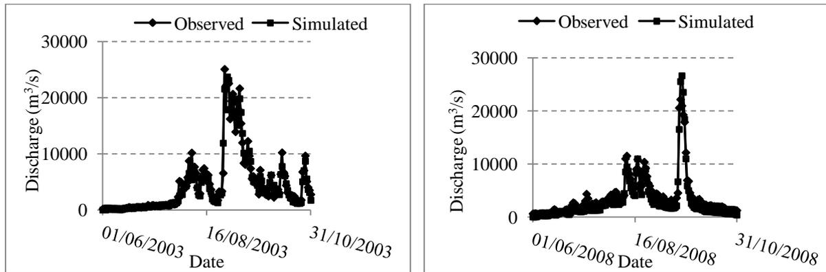
Fig. 5: (a) Calibration and (b) Validation of MIKE 11 HD Model
