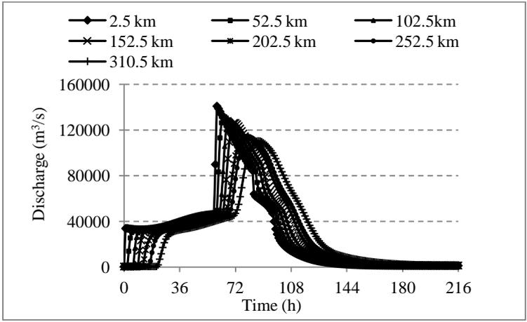
Fig. 9: Flood Attenuation Hydrographs of Dam Break Outflow at Different River Cross-sections
