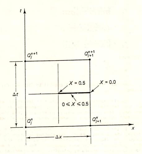
Figure 1. Space-time discretization of kinematic wave equation paralleling Muskingum method.
