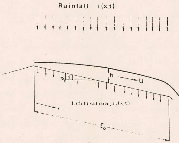
Fig 1 : Description of Overland flow on a plane
