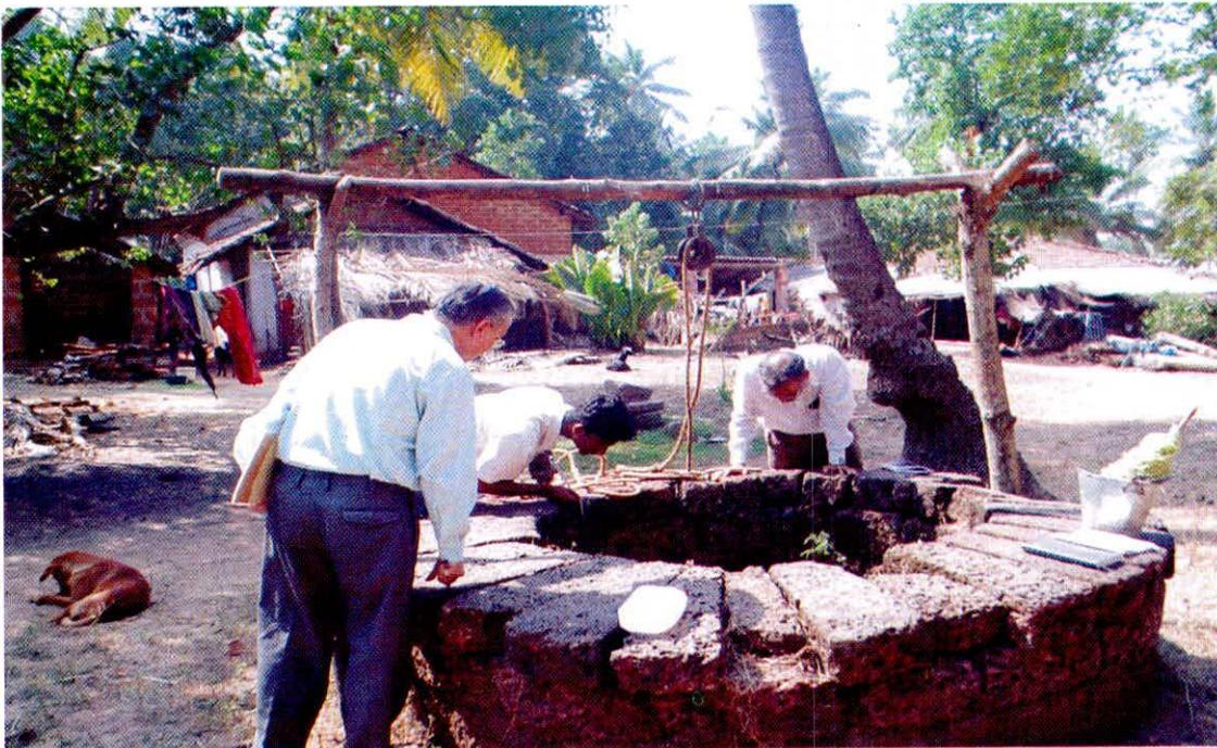
**Figure 9: Measurement of Groundwater Level in Observation Well Number 10**
