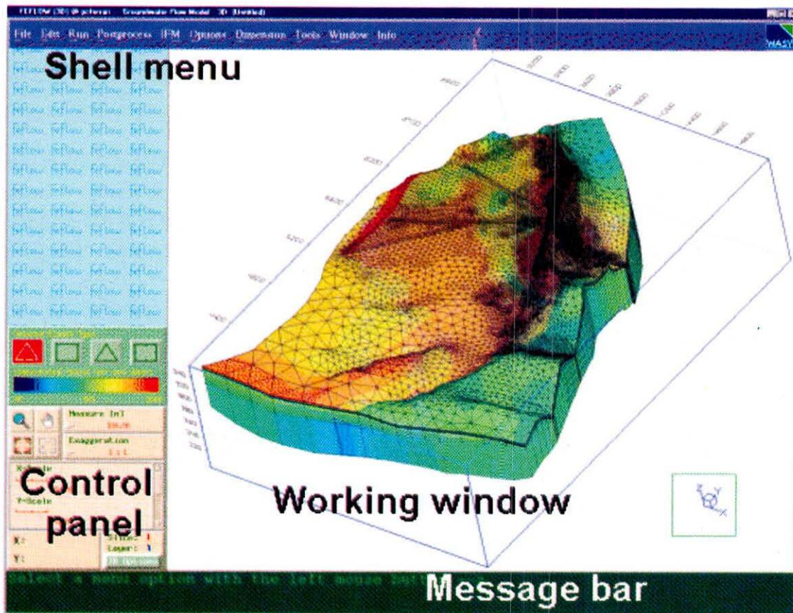
Figure 11 : FEFLOW Working Window
