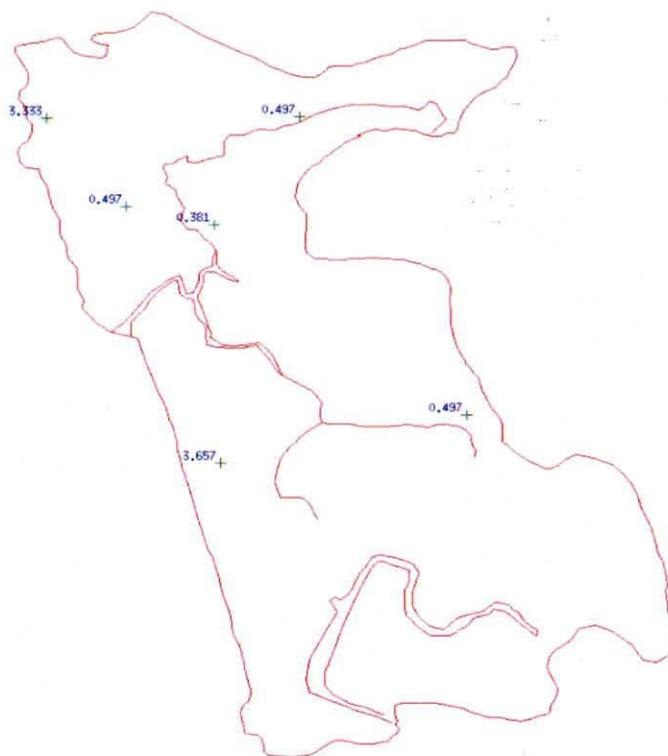
Figure 7: Measured Values of Hydraulic Conductivity ( $\times 10^{-4}$  m/s)
