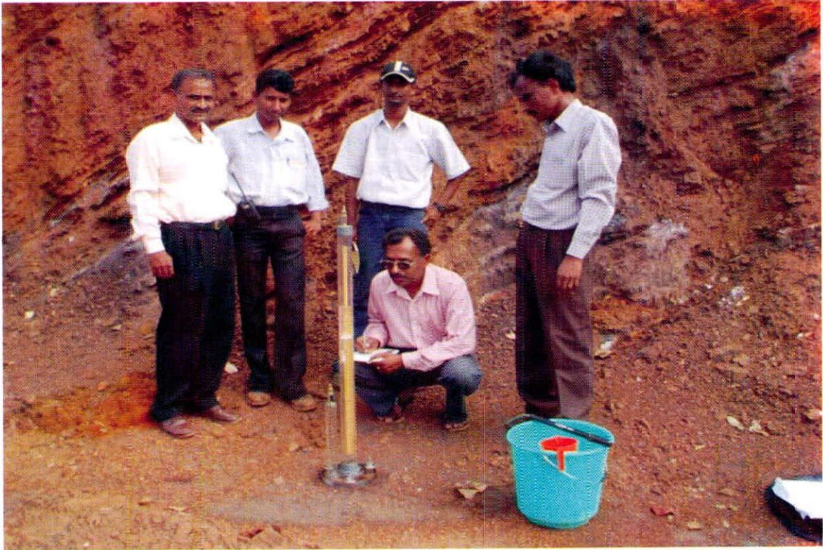
**Figure 10 : Measurement of Hydraulic Conductivity in Laterite Soil**
