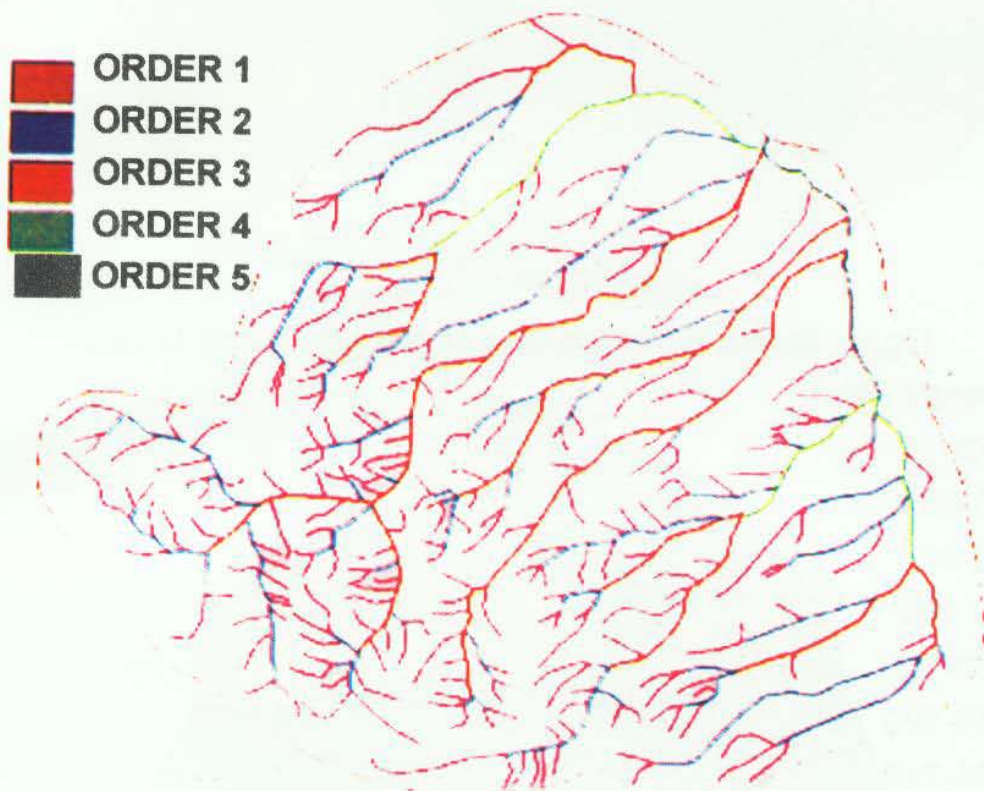
Fig.6-22 Drainage Network Map of Alnia Dam Catchment
