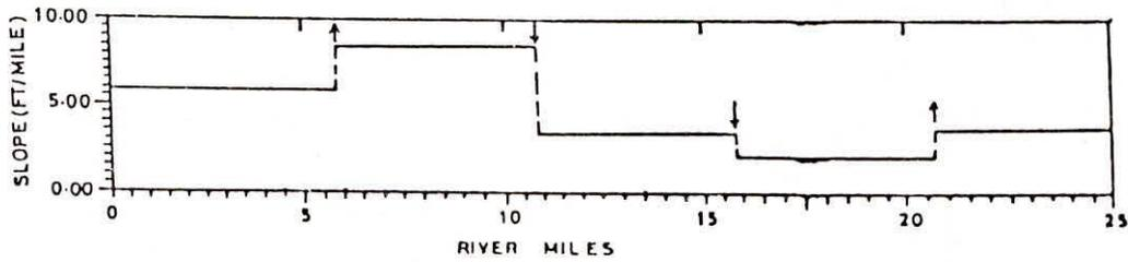
(b) BED SLOPE VARIATION ALONG THE RIVER VALLEY. UP AND DOWN ARROW MARKS INDICATE STEEPENING AND FLATTENING, RESPECTIVELY, OF ADJOINING DOWN STREAM REACHES.
