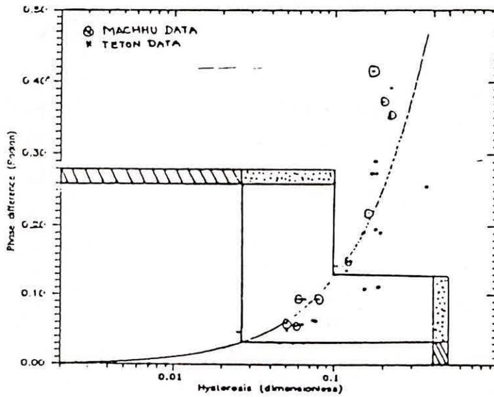
Fig. 7 : Dimensionless Hysteresis vs. Phase Difference (Radian) of Q & H -waves
