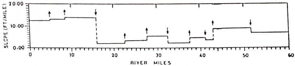
(b) BED SLOPE VARIATION ALONG THE RIVER VALLEY. UP AND DOWN ARROW MARKS INDICATE STEEPENING AND FLATTENING, RESPECTIVELY, OF ADJOINING DOWNSTREAM REACHES.
