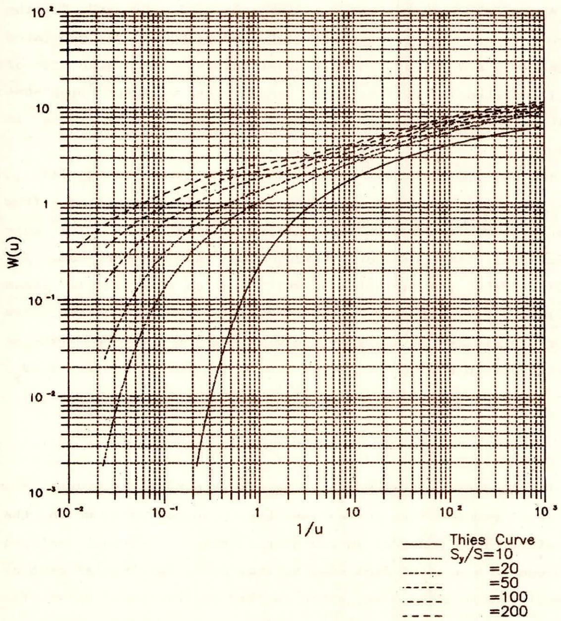
FIG.6 - Family of type curves:  $W(u)$  vs  $1/u$  for different values of  $S_y/S$ .
