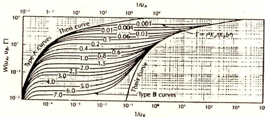
Fig.1- Neuman's Type Curve for Unconfined Aquifer without Delayed Yield
