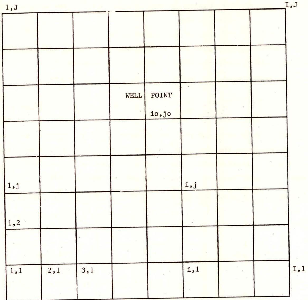
Fig. 4- Designation of grid nodes used in the derivations
