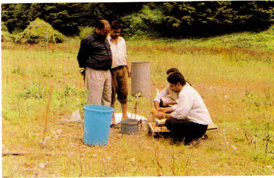
INFILTRATION TEST IN PROGRESS IN NAINITAL LAKE CATCHMENT, UTTAR PRADESH
