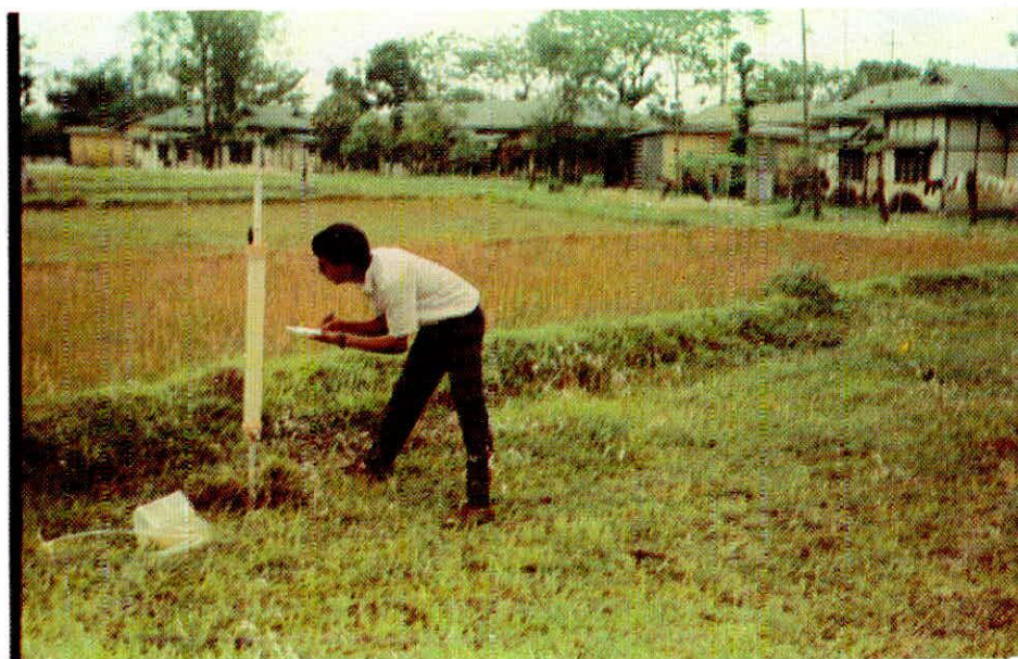
GUELPH PERMEAMETER BEING USED IN THE FIELD
