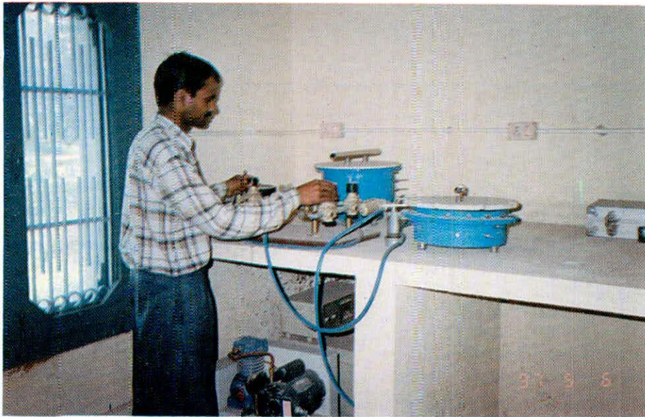
SOIL SAMPLE ANALYSES USING PRESSURE PLATE APPARATUS AT JAMMU REGIONAL CENTRE
