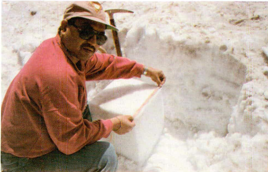
FORMATION OF A SNOWBLOCK FOR DETERMINATION OF SNOWMELT FACTOR
