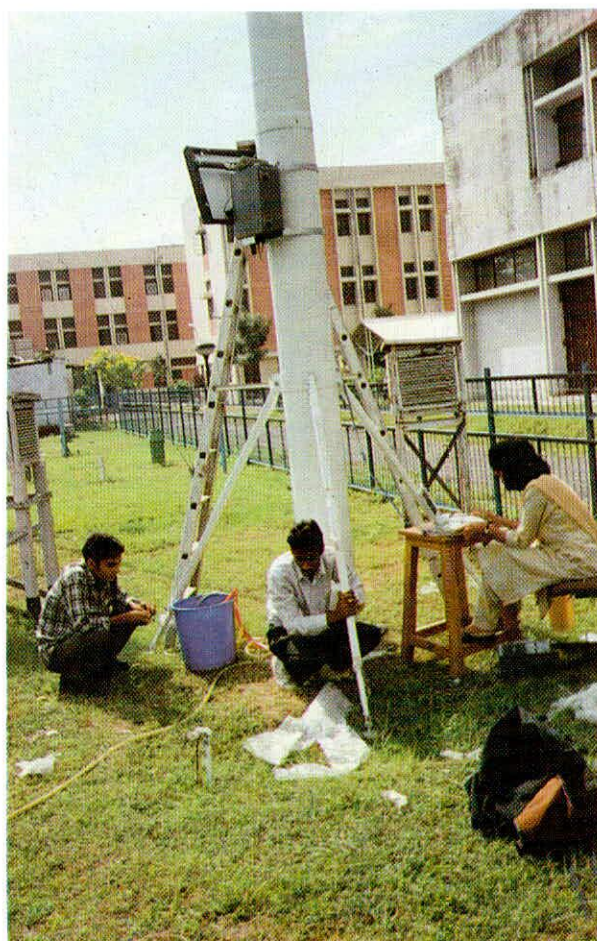
TESTING OF PRECIPITATION GAUGE
