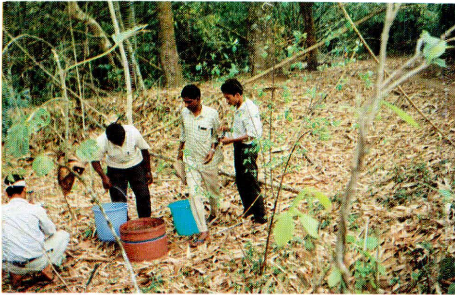
INFILTRATION TEST BEING CONDUCTED IN FIELD
