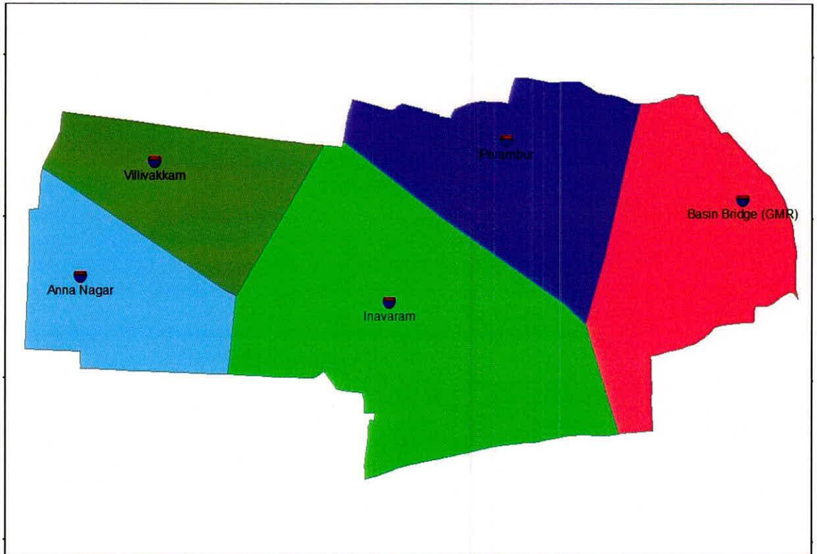
Figure 9. Map showing influence of each rain gauge using Thiessen Polygon method
