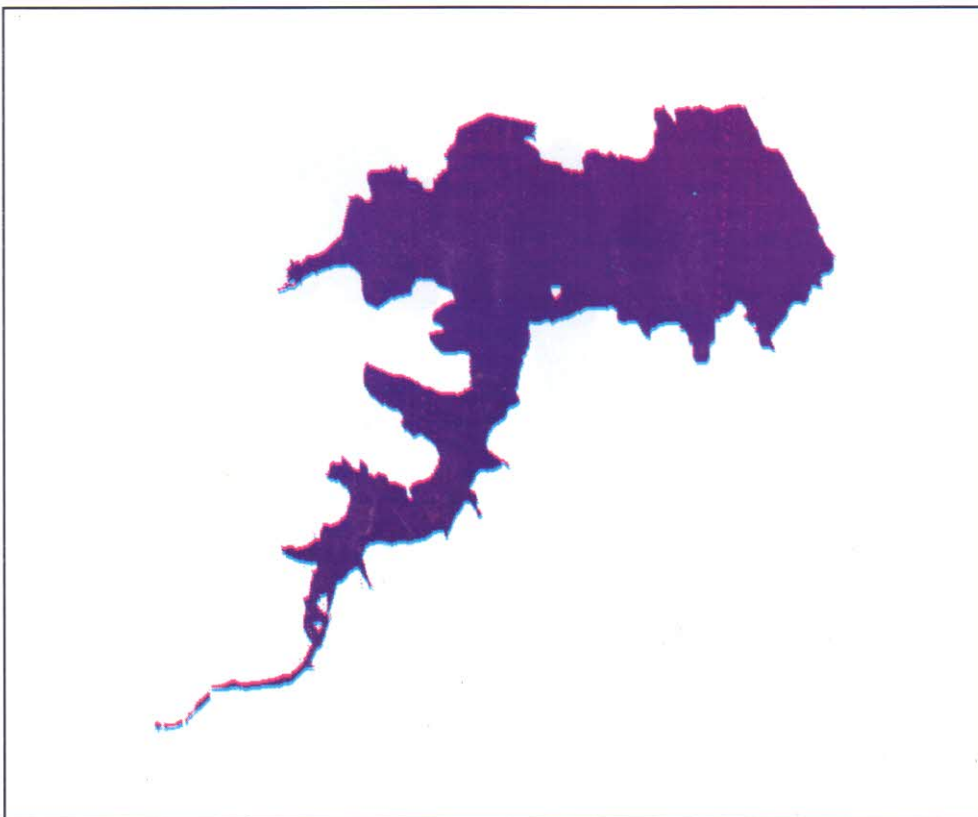
Figure 3.5: FCC of IRS 1 D LISS III data of February, 2001 and water spread area of the Ghatprabha reservoir
