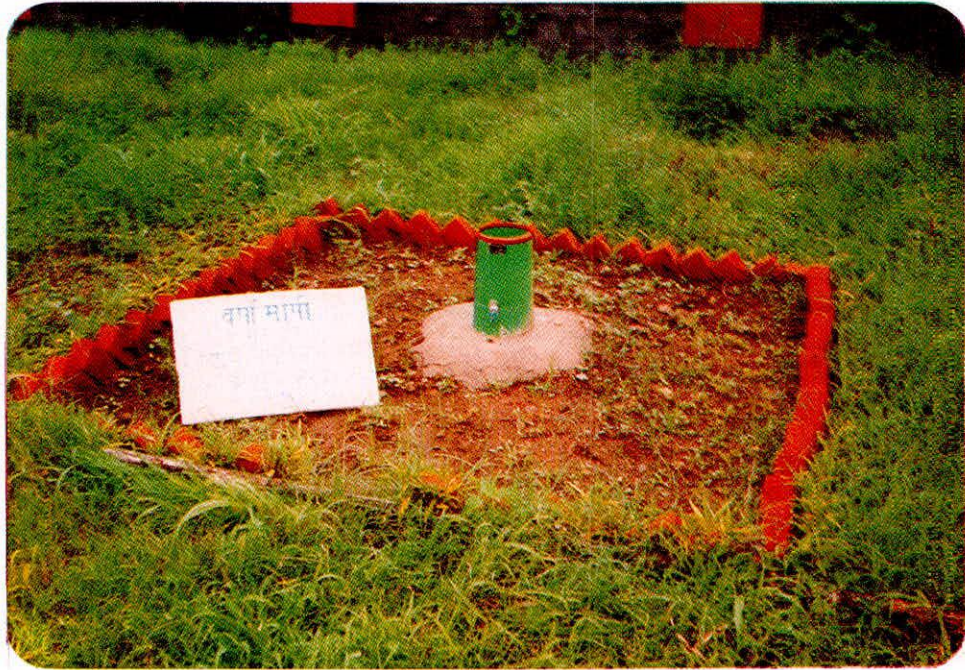
Raingauge Mahagaon Hard Rock Regional Centre, Belgaum
